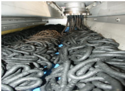
Figure 4.6. Sludge extrusion onto belt
